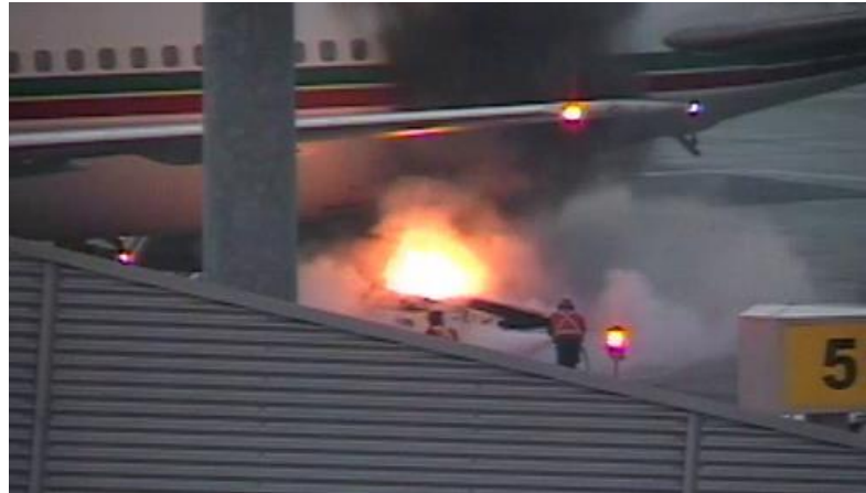
Photo 1. Ground crew trying to put out the fire with a wheeled dry chemical fire extinguisher (Source: Aéroports de Montréal)
