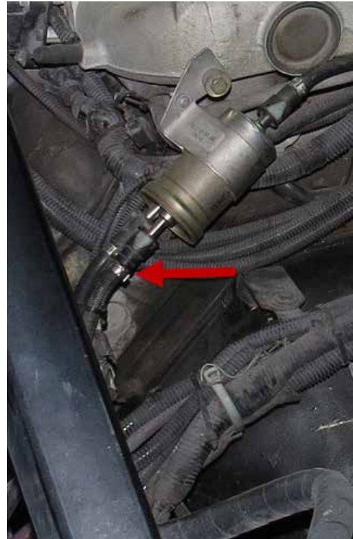
Photo 3. View showing crimped steel ring securing the connector of an identical, undamaged, belt loader
